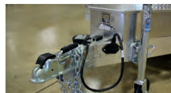
Lit Tool Box, Tongue Handle, and Receptacle Holder
